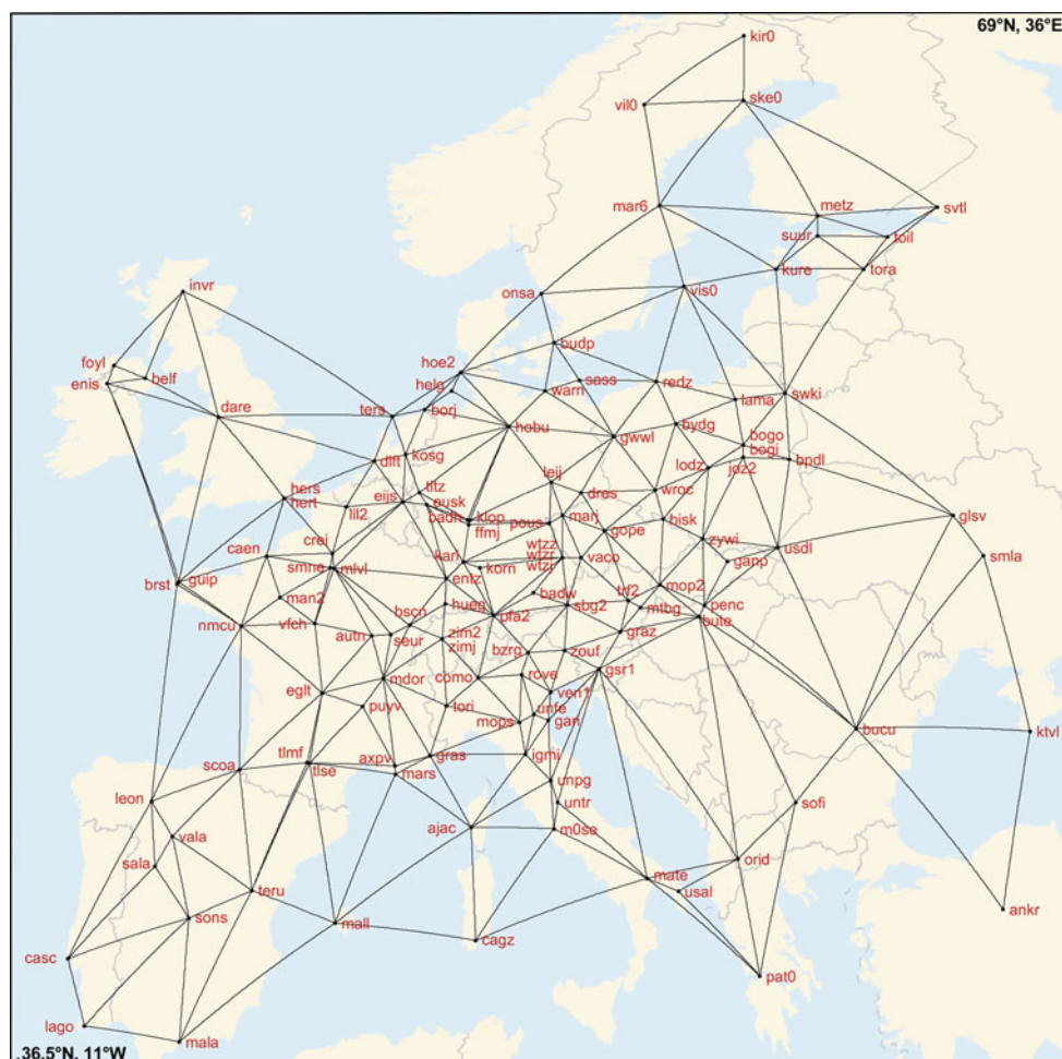
Fig. 1 Selected GPS/GLONASS reference stations in Europe and baselines used in the data processing
