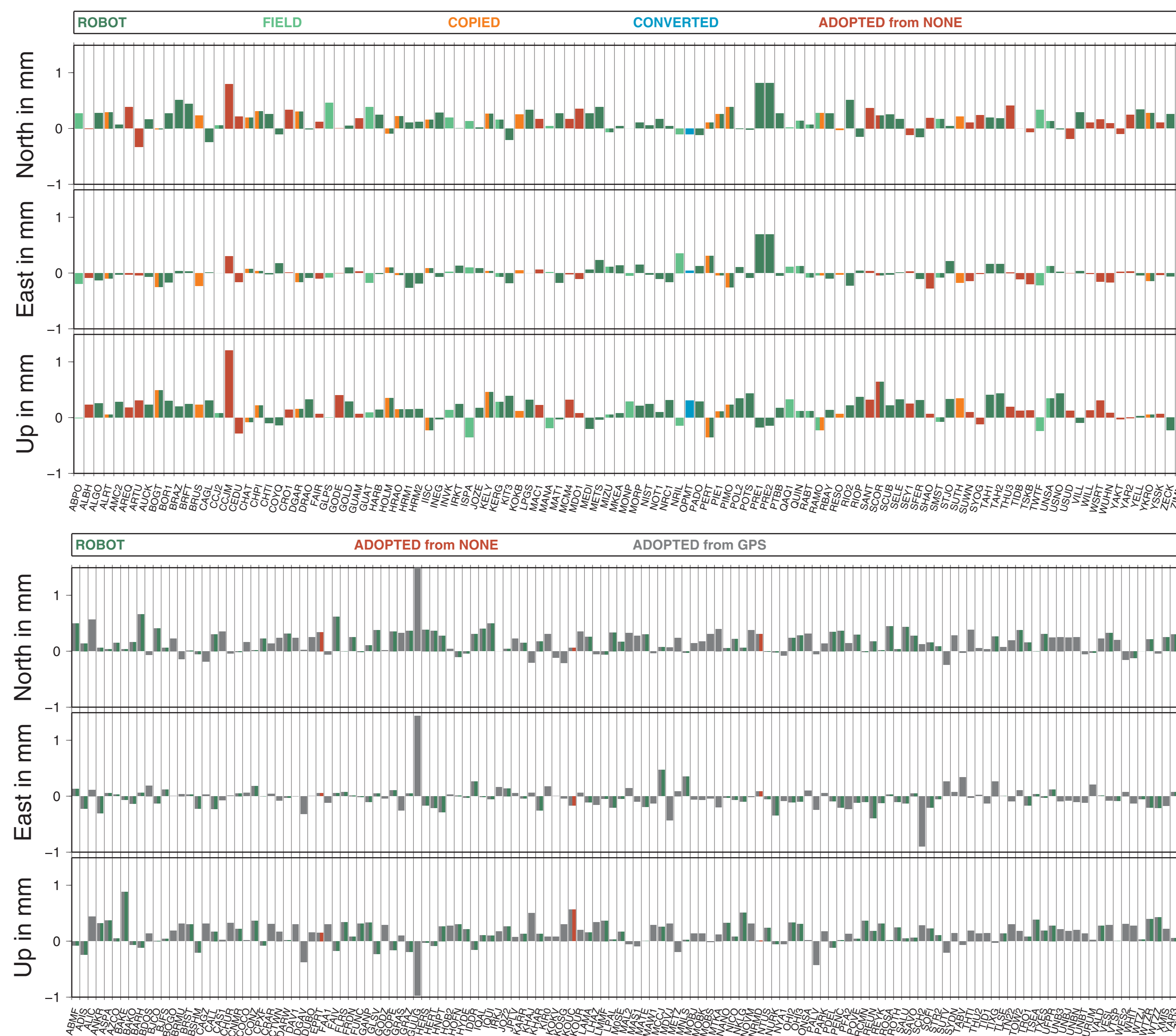
Figure 3: Change of the repeatability of the weekly coordinate solutions without estimating the GPS/GLONASS biases when switching from IGS05 to IGS08 modeling standards. A positive number indicates an improvement of the RMS of the coordinate time series. If the calibration method of an antenna has changes from igs05.atx to igs08.atx the bar is printed in two columns (left half indicating the calibration method from igs05.atx, right half from igs08.atx). The top plot refers to the GPS-calibration of the GPS-only stations, the bottom plot to the GLONASS-calibration of the combined GPS/GLONASS receivers. Overall, an improvement of the repeatability when switching from IGS05 to IGS08 is indicated, in particular for the north and vertical components. From the comparison of the two solutions it cannot be concluded whether it results from the introduction of system-dependent antenna corrections, from the increased number of ROBOT calibrated antennas, from the improved reference frame or from any other source.
