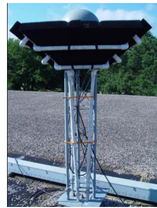
Fig. 7 Configuration of RF absorbing foam nest test case at the AUT site.
