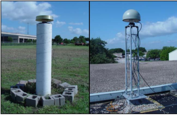
Fig. 5 Configuration of the choke ring-only (control) test case at the AUT site (right) and choke ring mounted at the REF site (left.) The REF site is only used for carrier phase analysis.
